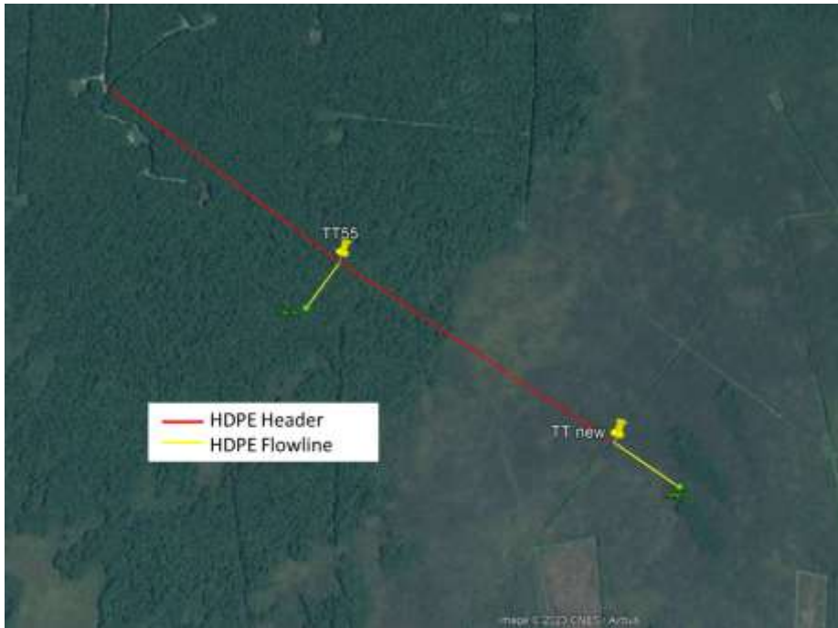
Figure 8: Routing of well 29PH07 and 29PD14 in the TNW South area
