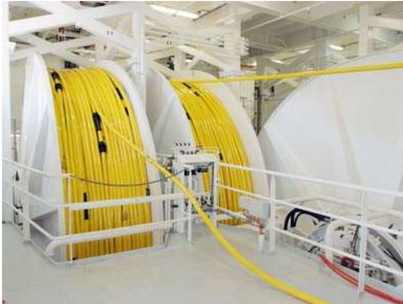
Figure 3: Solid Stream with sensitive hydrophones inside
