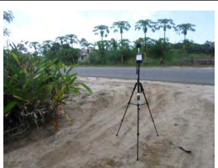
Location NU12: Driveway of the residence at the Wayamboweg. Nearest residence on the east side of the Soengie property. Distance from the axis of the road to the position of the noise meter is 8 m.
