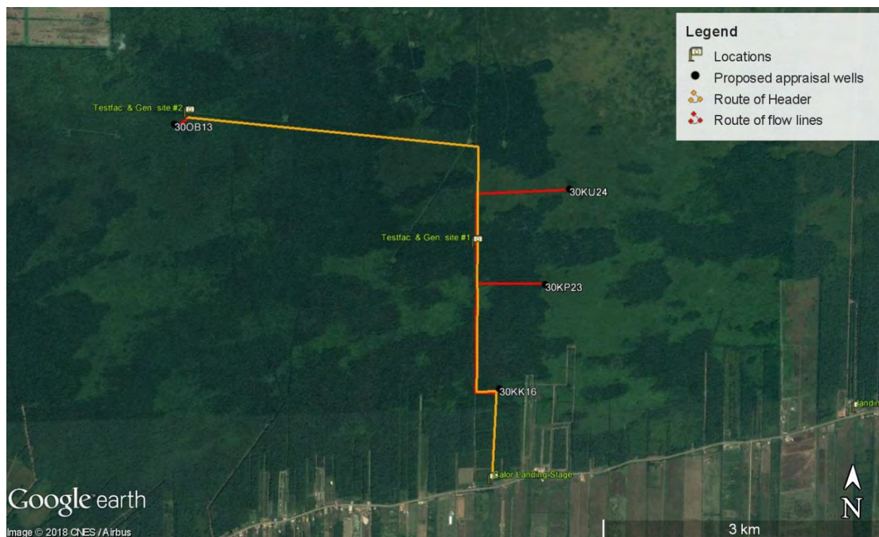
Figure 9: Overview of the route of the header to transport the crude oil from the test facilities to the collection tanks at the loading site
