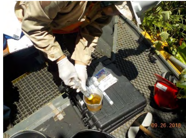
Location WQ-01: A syringe with filter (0.45u) used to filter the water sample for dissolved metal analysis
