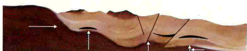
Continued uplift, followed by erosion. Folding and faulting. Accumulation of oil and gas in a sand layer.
