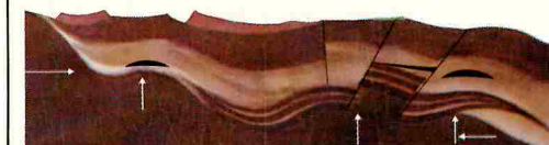
Continued uplift, followed by erosion. Folding and faulting. Accumulation of gas in a sand stratum.
