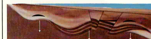
Subsidence and slight tilting. Renewed encroachment by sea. Sedimentation.
