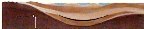
Basin practically filled. The sea recedes. Folding starts as a result of uplift and lateral pressure. Formation of oil and gas in layer of clay. Migration of oil and gas into a layer of sand.
