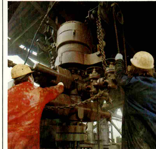
Every drill hole is provided with blow-out preventers which can be shut by remote control.
