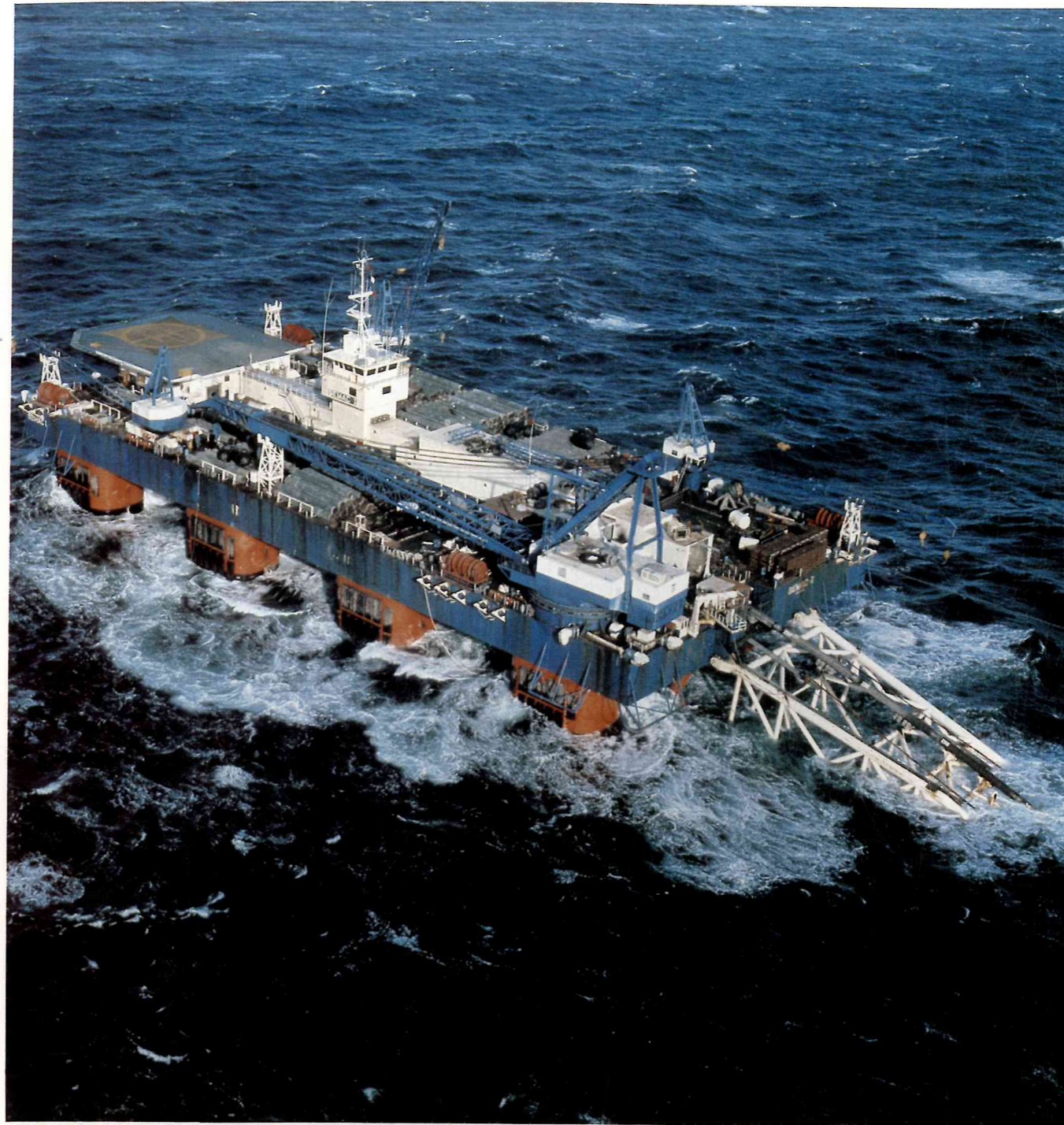
Left, Semac I, a semi-submersible pipe-laying barge, at work in the North Sea. Above, another pipe-laying barge, showing welded pipeline leaving the barge and passing down the stinger which guides the pipe towards the seabed.
