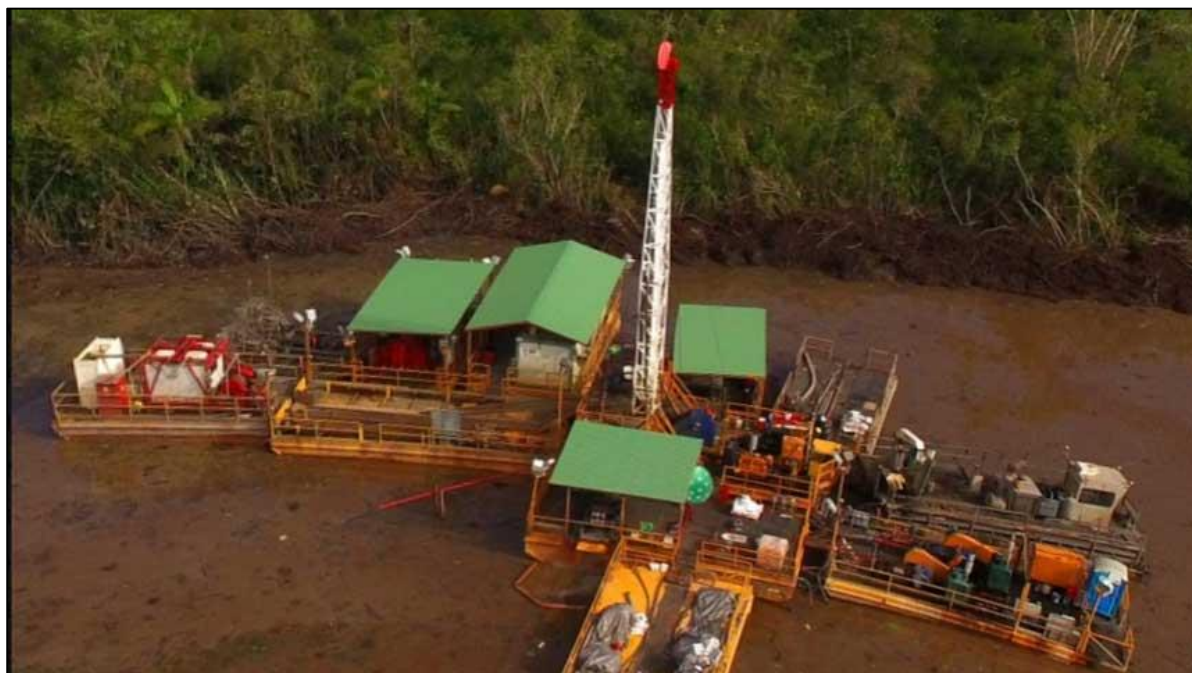
Figure 3-3: Swamp rig drilling a producer well in the Calcutta Oilfield
